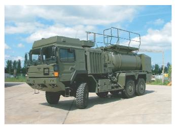
A 7,000 litre product tank mounted on a MAN Medium Mobility HX58 or Improved Medium Mobility SX44 chassis. These vehicles are constructed to European ADR and International Maritime Dangerous Goods regulations. They are equipped with 2 x hose reels discharging to the rear of the vehicle, bulk off-loading capability and are compatible with civilian fuel depot operations. Off road operations can be undertaken with these vehicles.
